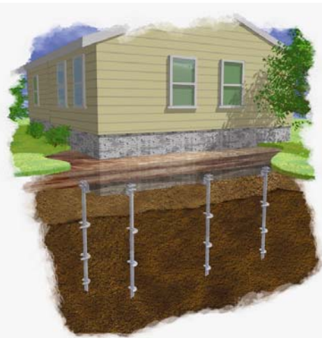
Helical piles will be drilled into the ground to support the foundations of two sinking buildings.
